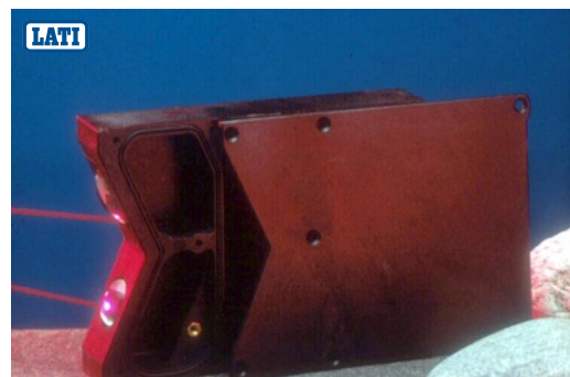
Housing for electronic instrument (used to measure the thickness of ceramic component) in LATISHIELD 87/28-07A G/20
