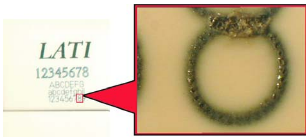
Fig. 15 LASULF white (PSU): darkening + slight foaming effect
