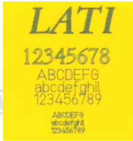
Fig. 18 LATER 4 G/15 yellow (PBT, Glass fibres): different quality of laser marking as a function of the pigment type used in the formulation
