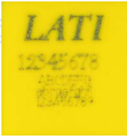
Fig. 18 LATER 4 G/15 yellow (PBT, Glass fibres): different quality of laser marking as a function of the pigment type used in the formulation
