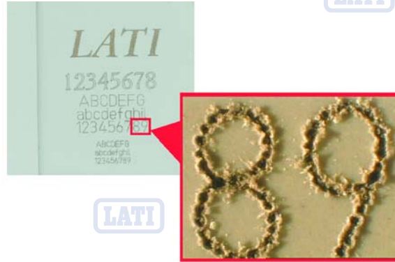
Fig. 14 KELON B FR H2 CET/30-V0 (PA6, mineral filled, FR with halogens): engraving + colour change. Visible engraved points at low magnification. At a normal distance the marking appears good readable.
